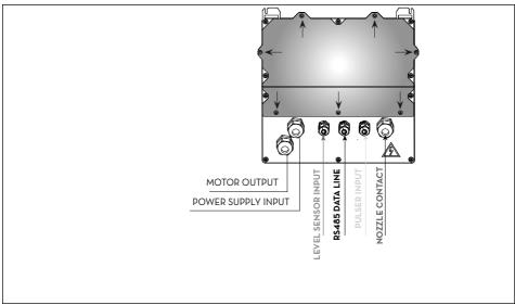
Once the cover has been opened, the electronic board and its connectors are accessible:
