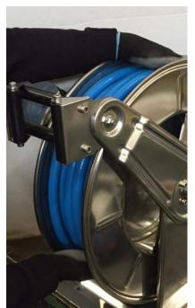
Let the reel rotate and download the spring charge ( obviously control the rotation)
