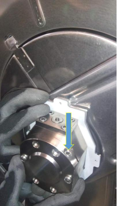
Put the brake on connection shaft.
