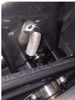
Hose reel must be positioned with ratchet armed and fixed on rack.
