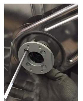
Take out the 4 screws with proper allen key
