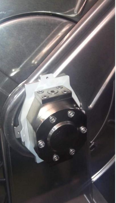
Tighten the four screws.
