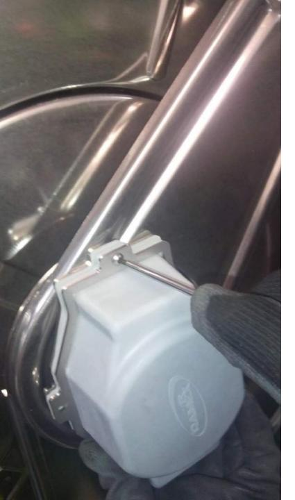
Fix the external frame adapter then tighten the four screws.
