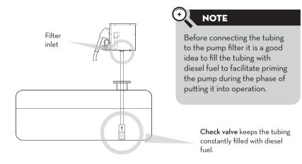
Connecting the hose to CUBE Screw the other end of the hose to pump filter.
