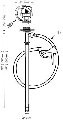
Engineered for transferring corrosive chemicals associated with the water treatment industry. Robust CPVC offers excellent durability and chemical resistance.
