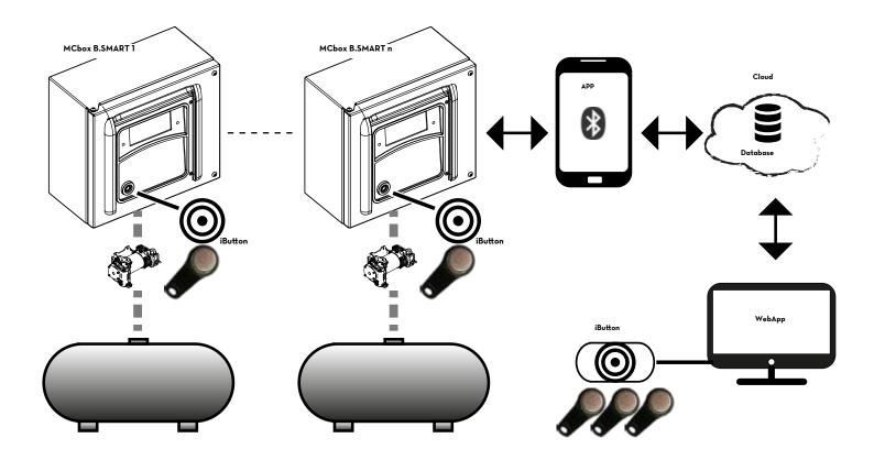
As can be seen from the descriptive diagram, each controller can manage 1 pump. There are numerous system configurations when using one or more controller. An example of the basic system structure is provided showing the possibility to:
