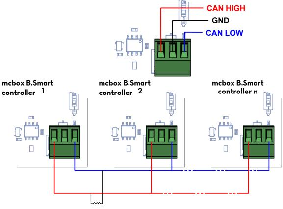
Insert the 120 ohm resistor provided between CAN HIGH - CAN LOW and connect the resistor output wires to the terminal boards, as shown in the figure.
