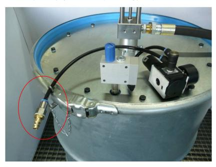
The cover is now ready for use. Compressed air can be connected.
