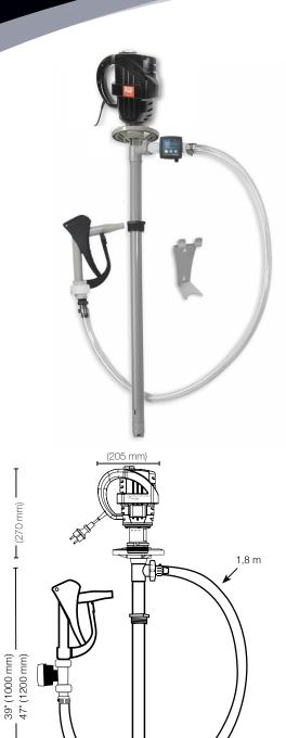
Engineered for transferring a variety of corrosive liquids. Robust Polypropylene ensures chemical resistance against light to aggressive chemicals. Equipped with a battery powered turbine flow meter for controlling, measuring and dispensing neutral liquids, corrosive chemicals (acids & alkalis) and many other non-flammable liquids.
