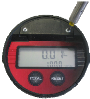
Picture 1: Loosen the battery cover
