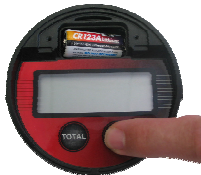
Picture 3: Insert the new battery and press the reset button to check the function of the register
