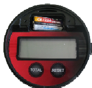
Picture 2: Take out the battery
