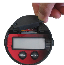
Picture 4: Insert the battery cover, then screw the battery cover tight
