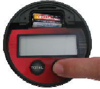
Picture 3: Insert the new battery and press the reset button to check the function of the register
